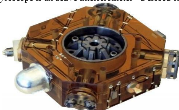
Fig. 2 Appearance of ring laser gyroscope
