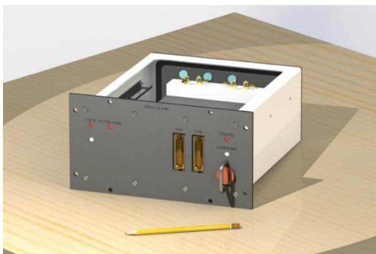
Fig. 1 External view of the unit for monitoring the parameters of microwave signals
