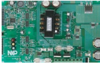
Fig. 3 JTAG/UART controller board
